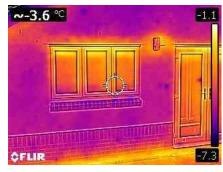
In a thermal picture, the lighter the colour, the greater the heat loss.
